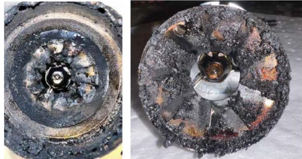
Figure B-6. Examples of retention heads with a rating of 5
