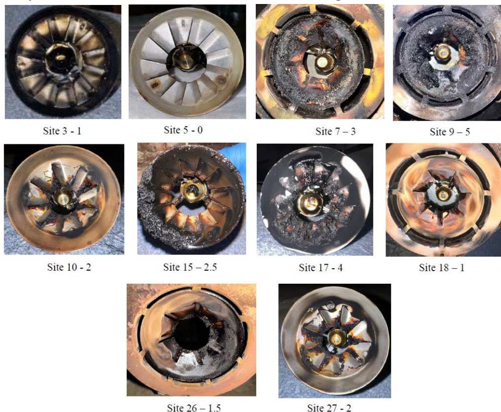
Figure 4. Photos of the retention heads from Level 1 sites with hot chamber boilers during visit period 5. The number after the dash indicates the coking level score.
