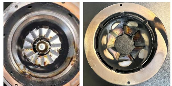
Figure B-2. Examples of retention heads with a rating of 1
